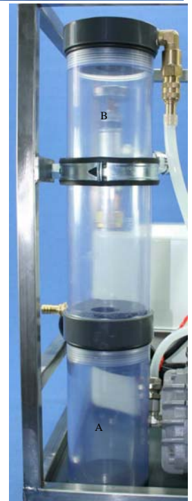
drying tower: A: condensate trap B: silica-gel stuffing
